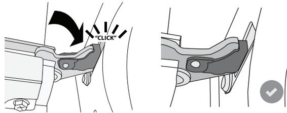
**5.** Try closing the door and check to make sure that it lines up with the control panel. If it does not, repeat the steps above: The door could become damaged if it does not work properly.
