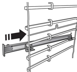
Remove the shelf guides from the oven and remove the protective plastic from the sliding runners.
