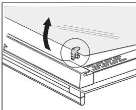
**3** The inner third glass (depending on the model) can be removed by lifting this carefully and removing it. Also remove the rubber seals around the glass.
