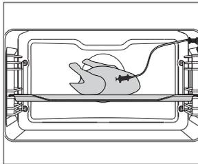
**2** Connect the meat probe plug to the socket and stick the probe into the food. (If any timer settings were activated, they will be cancelled.)
