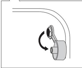
**1** Remove the cap (the socket is in the front upper corner of the oven right wall).
