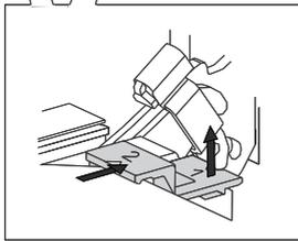
**1** Slightly lift the brackets on the left and right side of the door upwards (to marker 1 on the bracket) and pull this away from the glass slightly (to marker 2 on the bracket).
