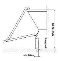
It is important to prevent the hose from coming loose and falling. For this purpose, the plastic support is equipped with a hole for tying it to the wall or water tap. The free end should be positioned at a height of between **30 and 100 cm**, and should never be submerged in water. If a horizontal drain extension hose is used (for a maximum 3 m), the drain hose can be placed at a maximum height of.**85 cm** from the ground.
