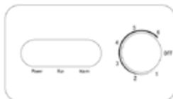
Set the appliance on a higher setting when the ambient air temperature rises to maintain the temperature inside the appliance.
